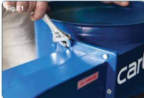
3. Attach the two collector support rods to the base plate with the four M5-0.8 x15 Phillips head screws, two flat washers and two hex nuts as shown.
